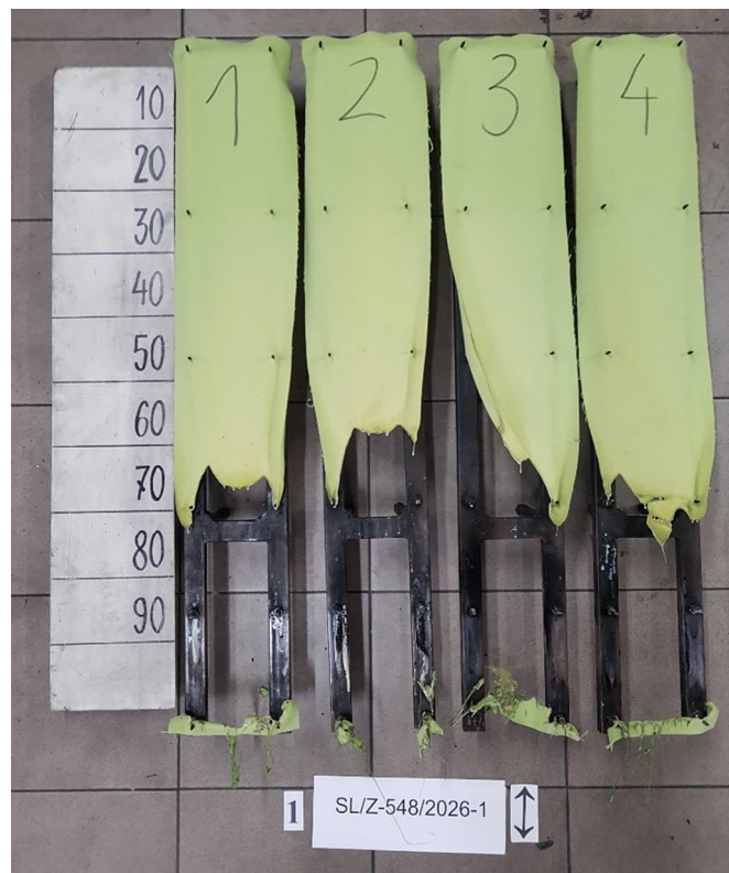
Figure 5. Appearance of the specimens 3 after the test - Light Colour: Apple, HYS096 Batch: 590188
