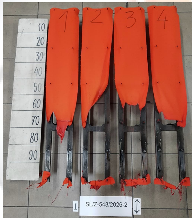
Figure 4. Appearance of the specimens 3 after the test - Medium Colour: Tortuga, HYS168 Batch: 584973
