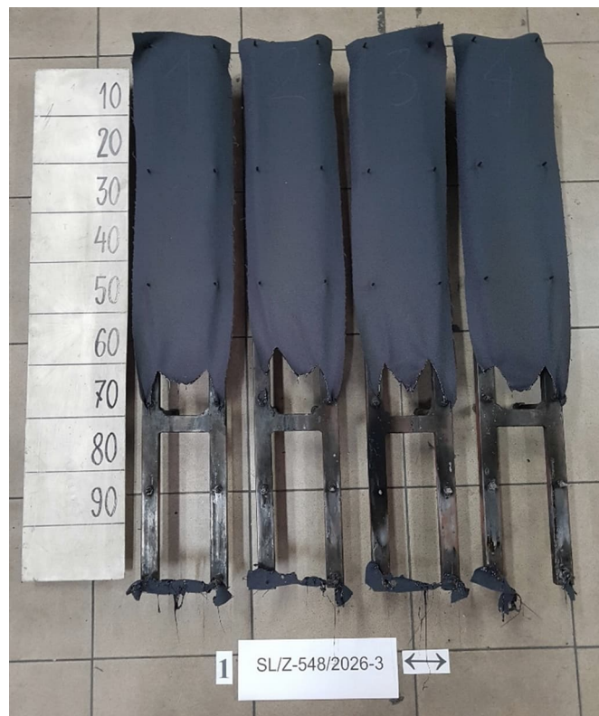
Figure 3. Appearance of the specimens 2 after the test - Dark Colour: Bonaire, HYS172 Batch: 589577, cross direction
