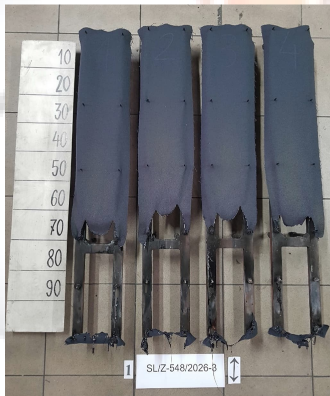
Figure 2. Appearance of the specimens 1 after the test - Dark Colour: Bonaire, HYS172 Batch: 589577, length direction
